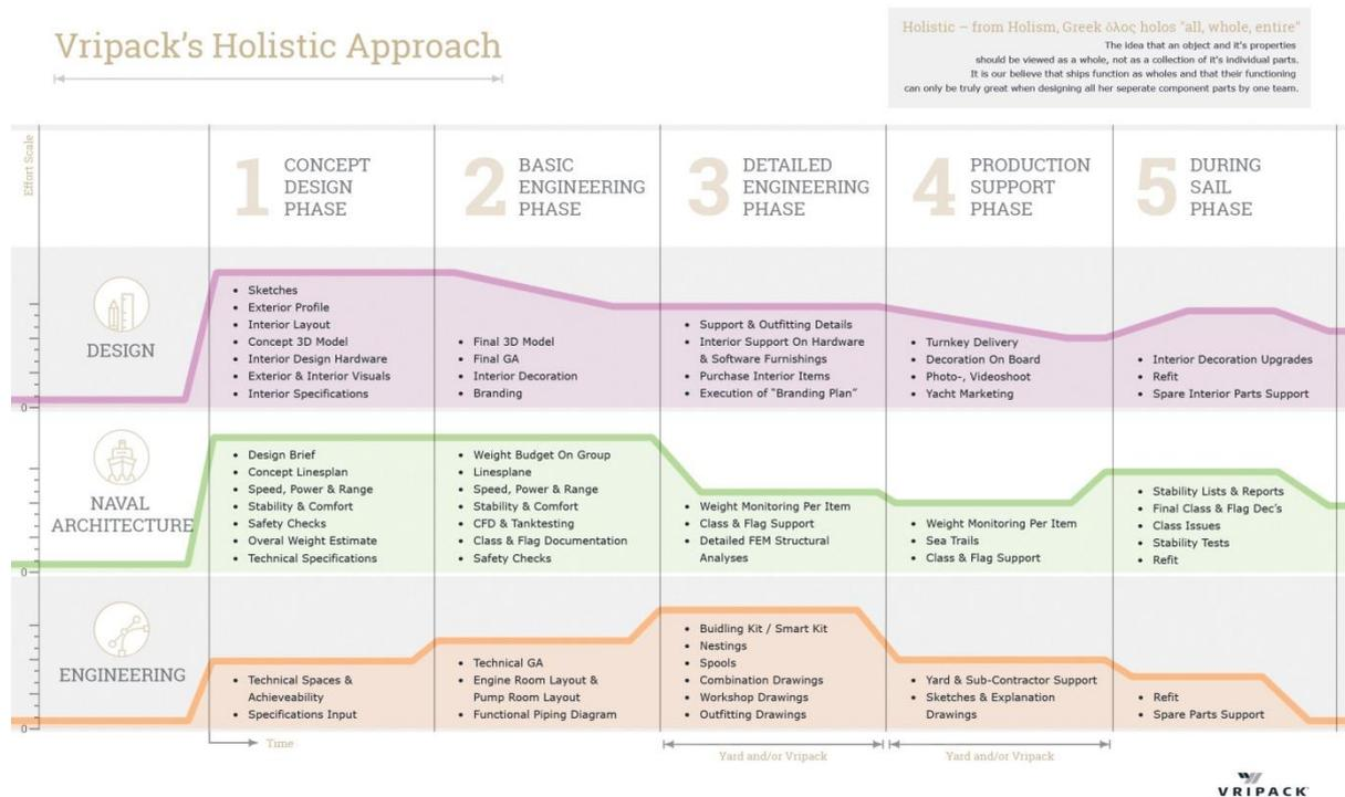
Fig. 1: Holistic Approach shows relationship between Design, Naval Architecture and Engineering
