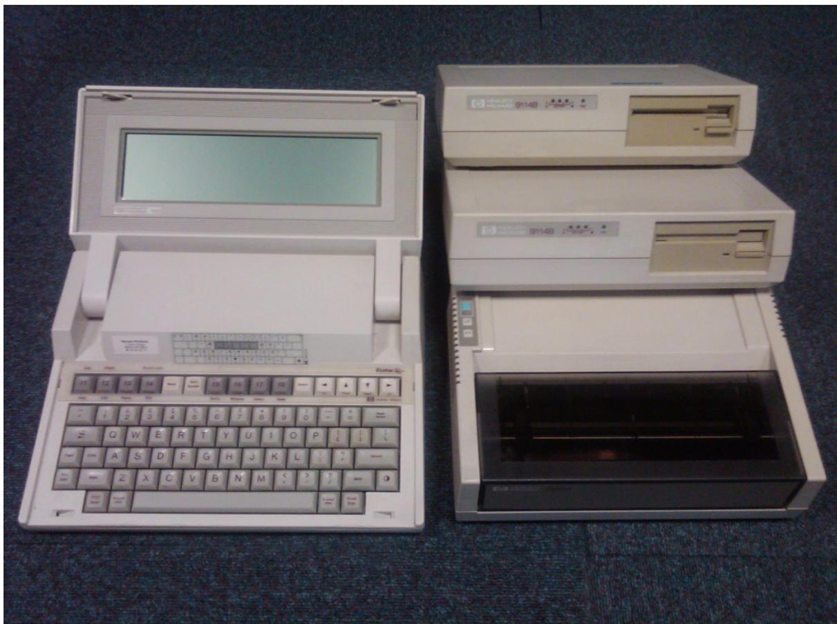
Fig.4: The HP110 second generation portable computer set includes ink-jet printer and portable disc drives for a total weight of under 4 kg and several hours battery autonomy,
