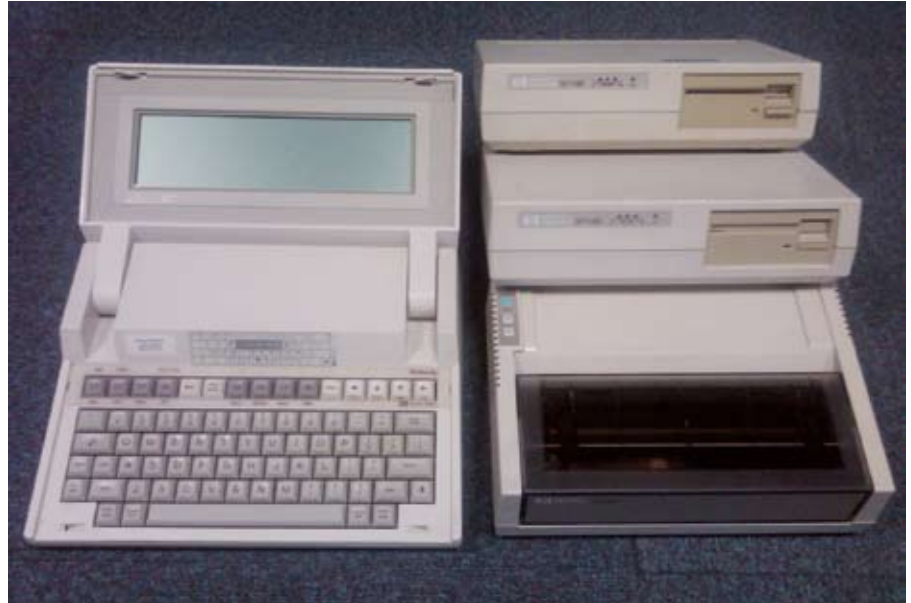
The HP110 second generation portable computer set includes ink-jet printer and portable disc drives for a total weight of under 4 kg and several hours battery autonomy
