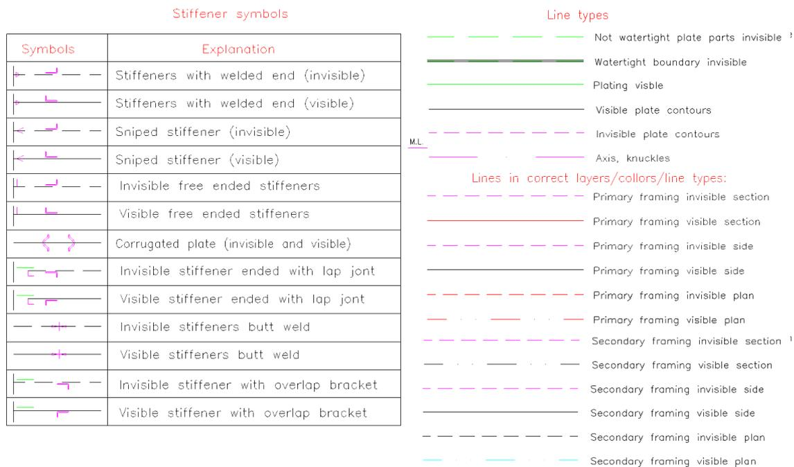
Fig.1: Example Standard Shipbuilding Symbols
