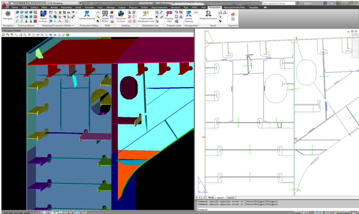
Fig.2: Profiles attached to plates as represented via ShipConstructor's MarineDrafting application
