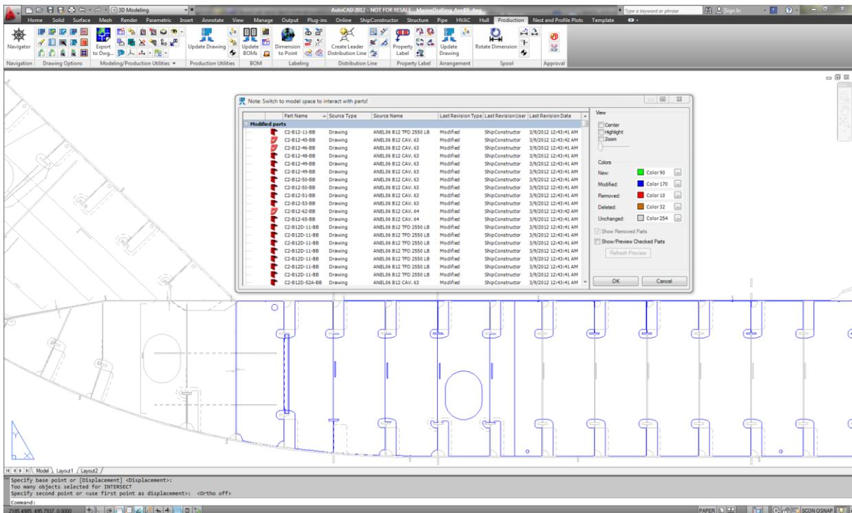
Fig.3: Change management within a MarineDrafting approval drawing
